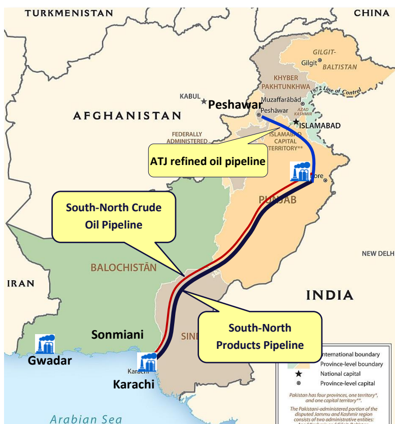
Figure 7.3 Planning Location of Oil Pipelines in Pakistan
